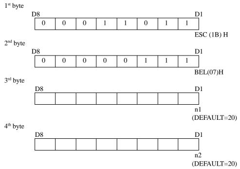
This command adjusts the drive pulse duration for the first drawer.
